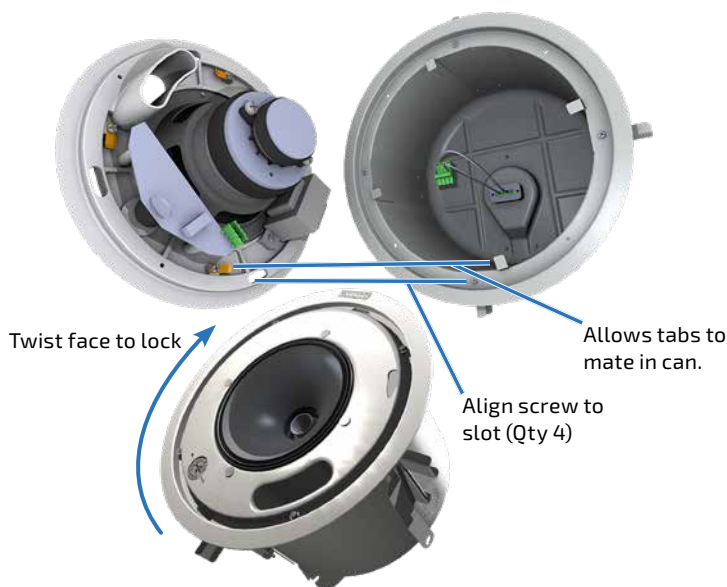
Figure 14. Four Twist-Assist™ face tabs inside the back can instantly secure the loudspeaker to the back can with a twist.
